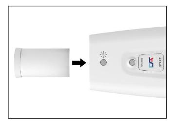
**Important:** Do not remove or replace the mouthpiece during UVC cleaning cycle, as indicated by a flashing UVC LED. Follow the instructions on the mobile app to know when to replace the mouthpiece.
