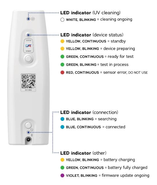
**Important:** If the LED indicator on the center of the device is showing red, do not use the device. Red color indicates that device sensors are not working correctly. Contact your local distributor for additional information.
